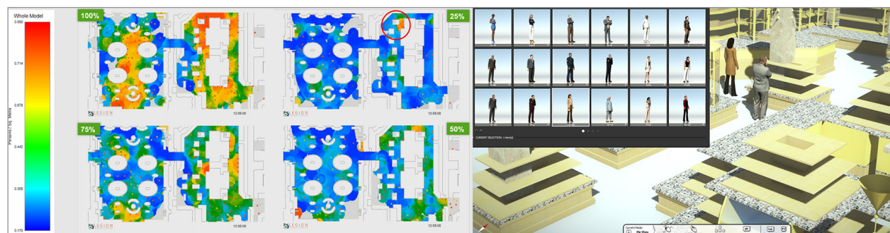
Figure 6. (Left) LEGION heat map simulation scenarios at 100%, 75%, 50%, and 25% occupancy models in a retail department store. (Right) LumenRT model showing socially distanced people placement in a retail department store and characters catalog.
