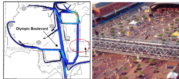
Figure 7. Congestion decreases on Olympic Boulevard with the adoption of the pedestrian footbridge over the rail tracks closing the circulation loop.
